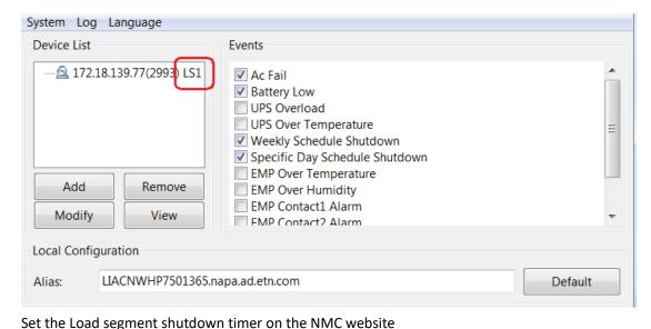
For example, the LS1 "shut down timer" is 180s and the LS2 "shut down timer" is 240s When the AC fail event occurs, the LS1 will be shut down after AC failing for 180s
