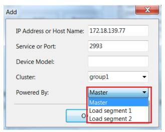
If the UPS support Load segment, you can choose LS1 or LS2. The device use LS1 as default. If the UPS don't support Load segment, you can use Master.
