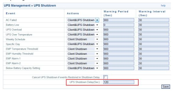
The UPS will be shut down after the "Warning Period" plus "UPS Shutdown Delay", if the action is "Client &UPS Shutdown".
